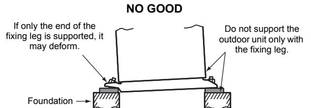
Set the out margin of the anchor bolt to 15 mm or less.
