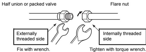
2. As shown in the figure, be sure to use two wrenches to loosen or tighten the flare nut of the valve on the gas side. If you use a single crescent, the flare nut cannot be tightened to the required tightening torque. On the other hand, use a single crescent to loosen or tighten the flare nut of the valve on the liquid side.
