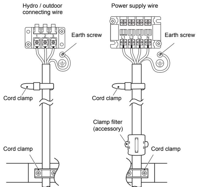
**Stripping length power supply wire and system interconnection wire**
