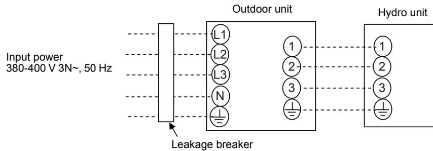
For the air to water heat pump, connect a power wire with the following specifications.
